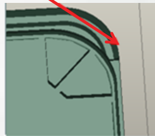
Reinforcement ribs on keyboard bezel corners
